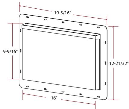
Note: Flange is pre-cut. On-site fabrication is necessary to accommodate penetration opening(s).
